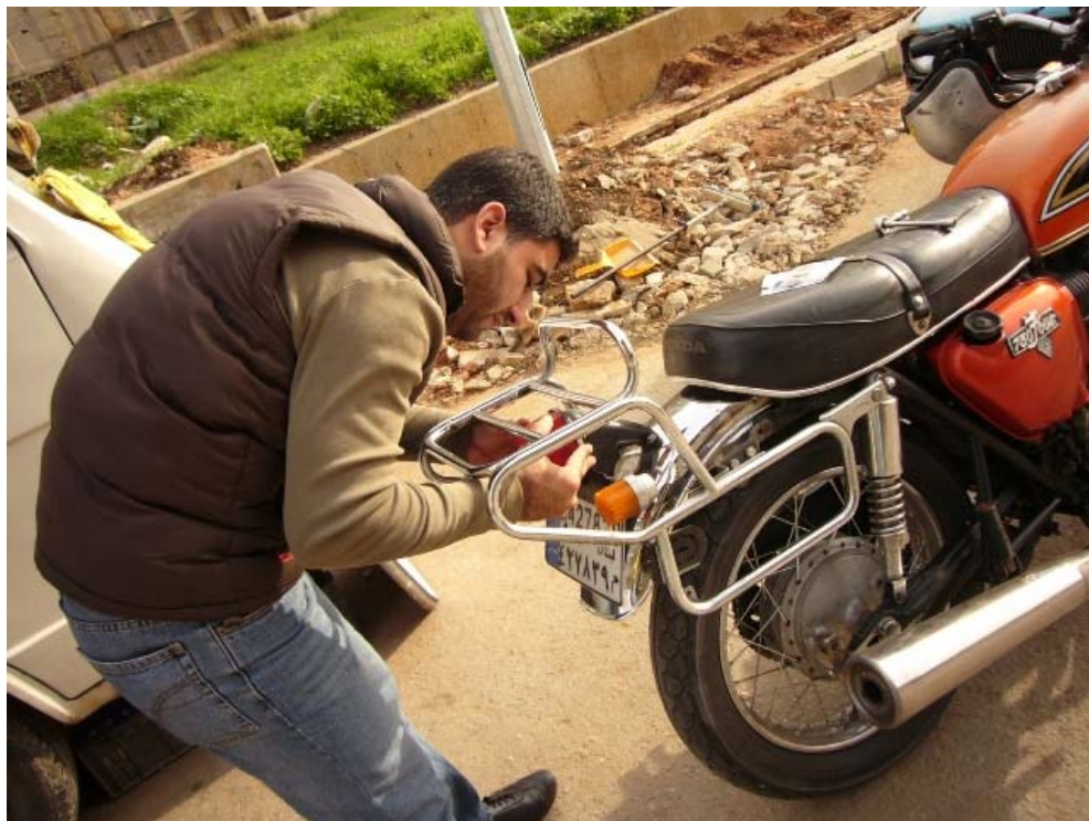
Basem installs a red brake lamp temporarily. The K6 passes the 2 nd inspection, then we put the original orange lamp back...
