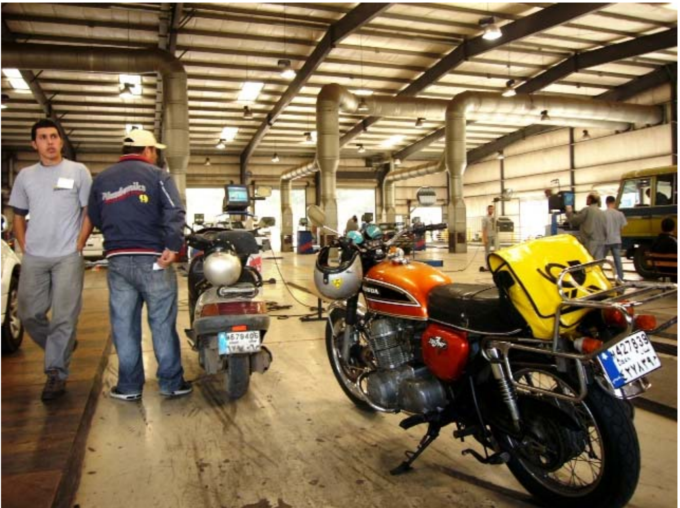
Official technical inspection: The K6 fails because of the original orange brake light in the back! In Lebanon, it should be red.
